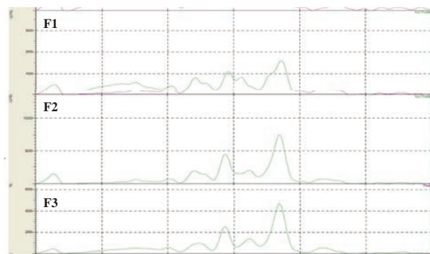
Figure 8. Results of X-ray diffraction for the MMEO-PEG 4000 solid dispersion:F1 = Solid dispersion by comparison MMEO:PEG 4000 (1:1 w/w); F2 = Solid dispersion by comparison MMEO:PEG 4000 (1:3 w/w); F3 = Solid dispersion by comparison MMEO:PEG 4000 (1:5 w/w).
